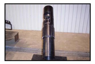
The valve assembly is now ready to be pressure tested. It is recommended that, with the lower valve fully open, the upper valve be cycled open and closed. Then, with the upper valve fully open, visually inspect the internal diameter of the valves with a flashlight to confirm that the balls of both the upper and lower valves are in the fully open position.
