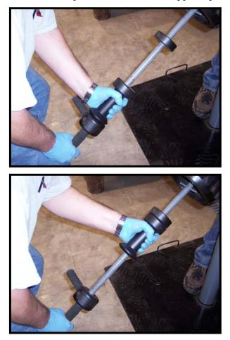
10. Use the slide handle to tap the canister into the upper top drive body seal bore.
