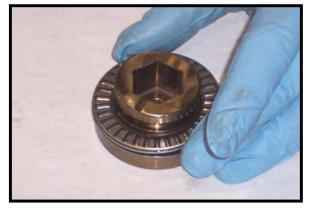
and (3) placing the second thrust washer on the stem.
