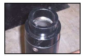
8. With the positioning tool in the vertical position, set the closed canister over the cap and rotate until the canister sits down on the two positioning pins located on the insertion cap. This places the canister stem links, which engage the stems, in line with the indicator handle at the bottom of the positioning tool.
