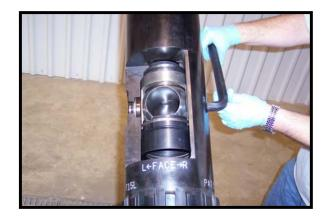
5. Using the slide handle on the positioning tool, hammer in a downward direction to remove the canister from the upper valve. The positioning tool handler should be prepared for the canister to disengage from the valve and remain attached to the top of the positioning tool. Further, care should be taken, as the canister will fall from the upper valve body if not fully engaged with the positioning tool upon removal.
