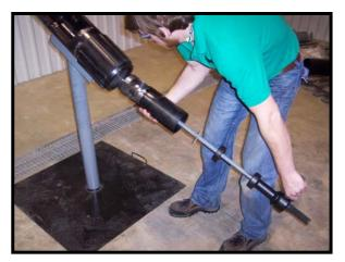
At this point, the operating stem assemblies can be removed for redress if so desired. The crank-arms would need to be removed if redressing the stems. With the canister removed, the operating stem assemblies can be removed. The stem assembly consists of the stem, stem o'rings, and two thrust washers with a thrust bearing between them. It is imperative that all these parts are retrieved from the valve and are accounted for. To remove the operating stem assembly, this step must be followed:
