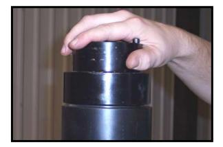
2. With the male threads of the positioning tool exposed, insert the positioning tool into the upper valve through the internal box connection.
