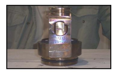
15. Slide the ball in between the cage legs ensuring that the ball slot aligns with and engages the back portion of the stem link(s)
