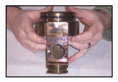
10. Lubricate the cage bore.
