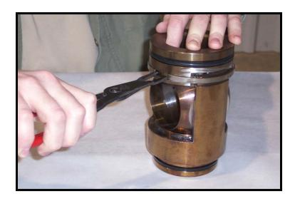
2. Slide the cage/seat fastener out of the cage/seat grooves on the canister and remove the top seat from the cage.
