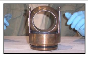
16. Insert the cage/seat fastener into the cage/seat fastener groove on the upper seat.
