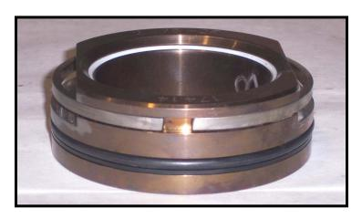
17. Place the upper seat on top of the cage legs. Align the upper seat flats with the cage legs.
