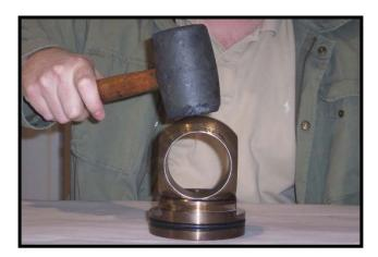
8. With the lower seat on a flat surface and the Teflon groove facing upward, place the ball on the lower seat. Ensure that the internal diameter of the ball is perpendicular to the lower seat and that the Teflon ring is completely covered by the outside diameter of the ball. Using a rubber mallet, tap the ball with moderate force to ensure that the lower seat Teflon ring is seated.
