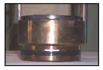
14. Insert the stem link vertically into the cage window. If assembling a dual window canister, insert one stem link into each of the two windows.
