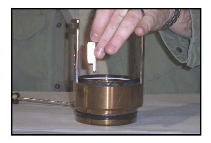
5. Remove the lower seat from the cage bore.
